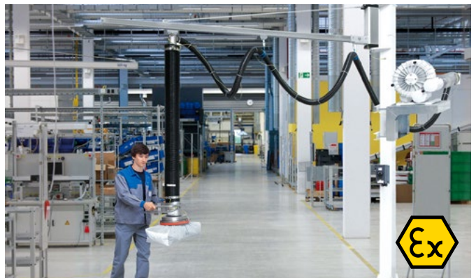
ATEX JIB CRANE FOR POTENTIALLY EXPLOSIVE ATMOSPHERES
