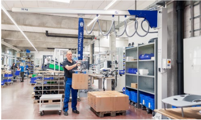
ALUMINIUM FLAT JIB FOR PARTICULARLY LOW CEILING HEIGHTS
