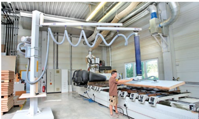
TELESCOPIC JIB FOR HARD TO ACCESS WORKING AREAS
