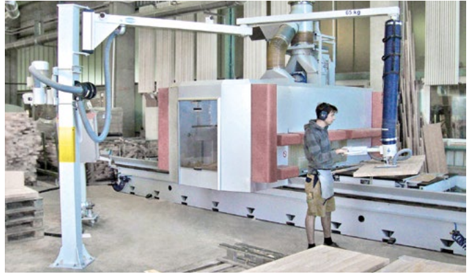
ARTICULATED ARM JIB FOR CIRCUMVENTING INTERFERENCE CONTOURS
