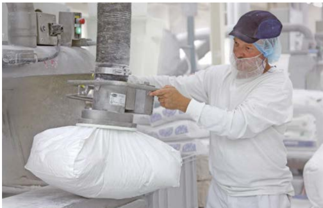
Vacuum tube lifter JumboSprint Ex for handling bags in an explosion protection zone
