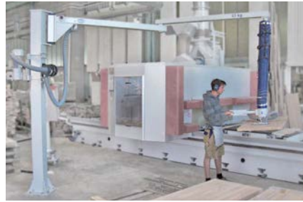
Articulated-arm jib to move around obstacles
