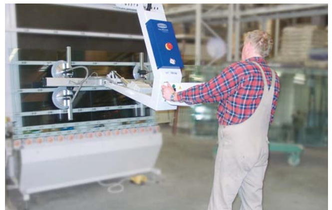
Vacuum lifting device VacuMaster Comfort for turning a glass sheet by 180°
