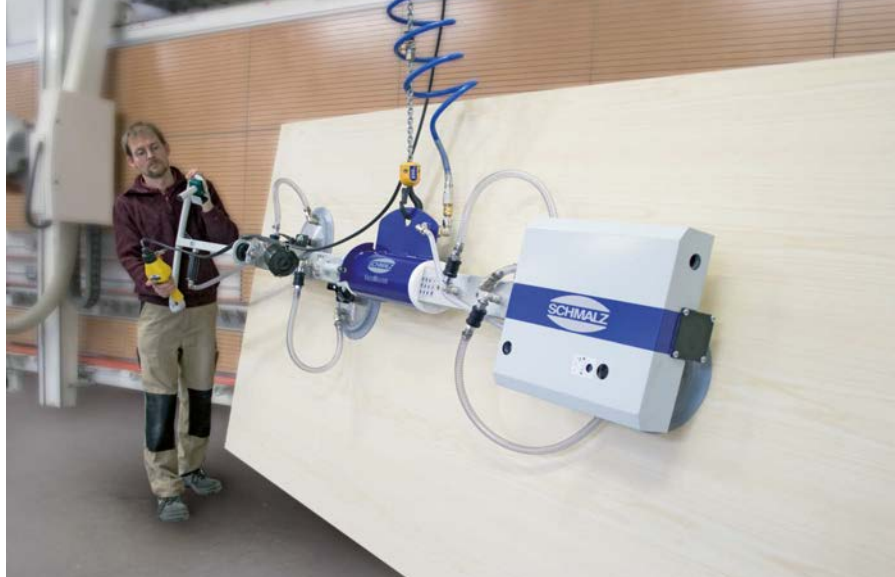
VacuMaster HHVM for removing wooden boards from upright storage
