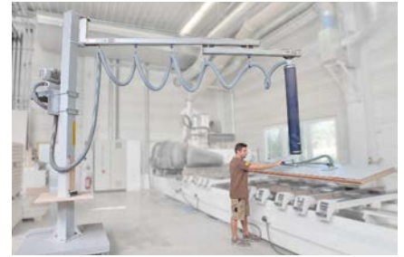
Telescopic jib for confined working areas
