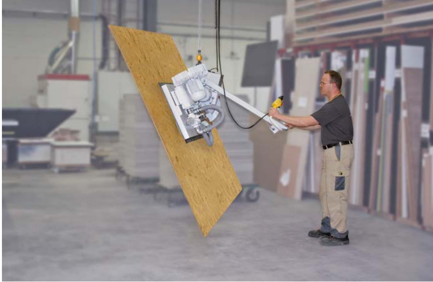
VacuMaster Multi for swiveling wooden boards by 90°
