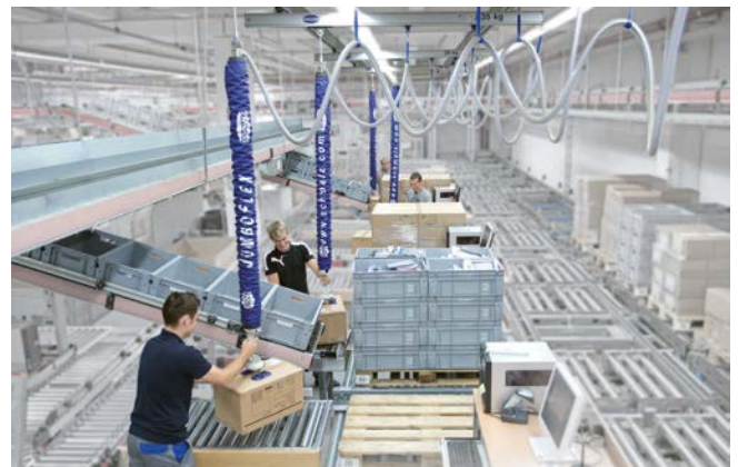
Vacuum tube lifter JumboFlex for handling packages in goods receiving/shipping
