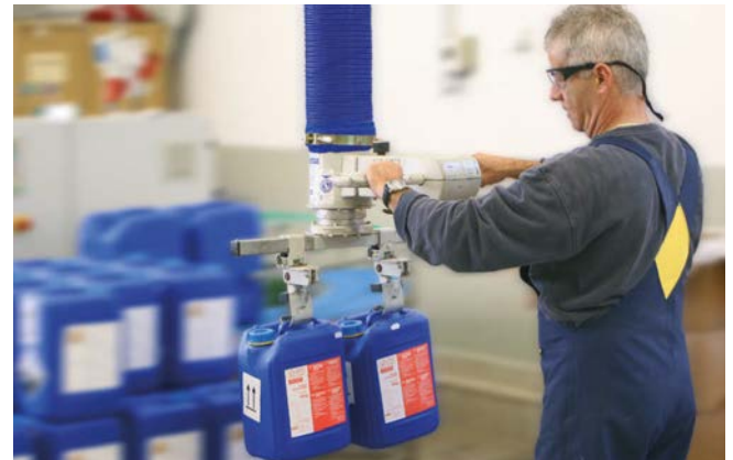
Vacuum tube lifter JumboErgo with mechanical gripper for handling jugs
