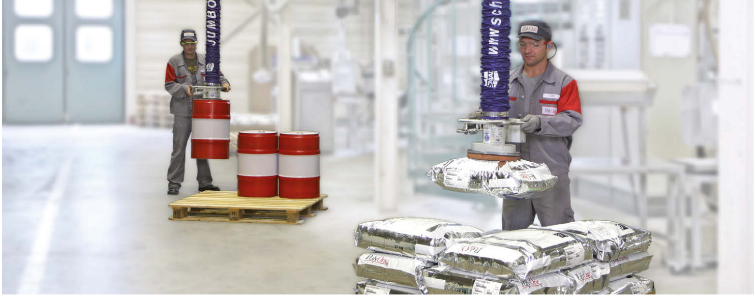
Vacuum tube lifter Jumbo Sprint for palletizing barrels and bags
