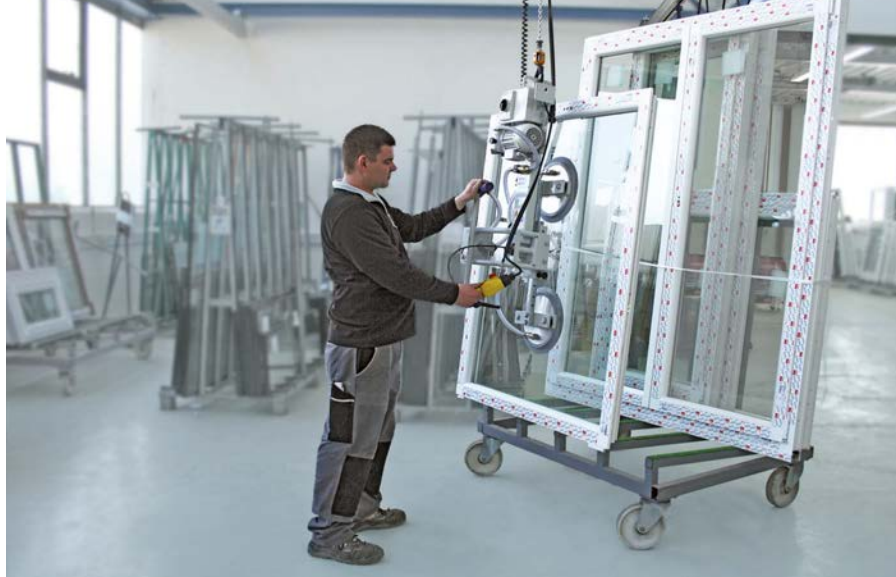
VacuMaster Window for rotating and palletizing windows
