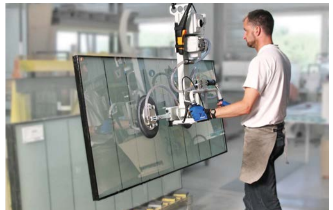
Vacuum lifting device VacuMaster Window for vertical handling of glass elements
